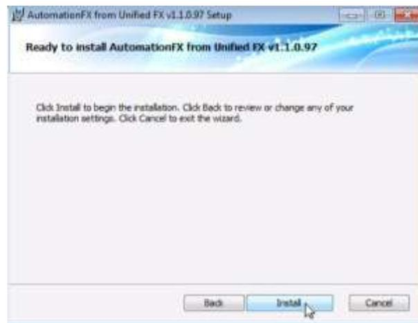
All necessary files will then be copied to the local machine and the AutomationFX Windows Service will be installed and started.
